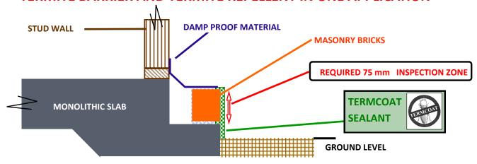
The purpose of Modern Physical Termite Management Systems is to force Termites to the external exposed perimeter of the building to allow for visual detection of termite migration into the structure as evidenced by a minimum of 75mm of termite mud tube over the visual inspection zone.
